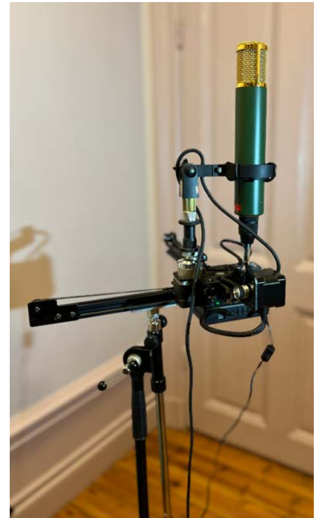
Robot for comparison of dynamic, frequency, and directional responses of different microphones
